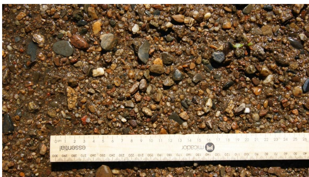
Figure 11. Bed load sediments from the Gigerline Reach which are predominately coarse gravels.
