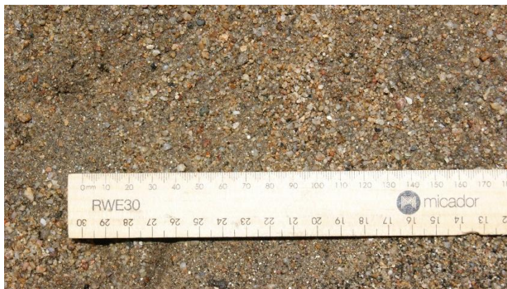
Figure 9. Typical composition of the bed load of the Tharwa reach of the Murrumbidgee River (Photo: Ben Broadhurst)
